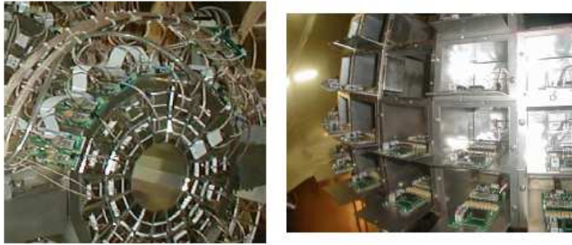
FIGURE 4.8: Photo of the motherboards placed on the external surface of the wheels mechanical structure (left) and on the top of the metallic baskets for sphere detectors (right)[76].
