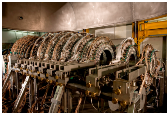
FIGURE 4.2: Photo of the CHIMERA multidetector placed at INFN-LNS.
