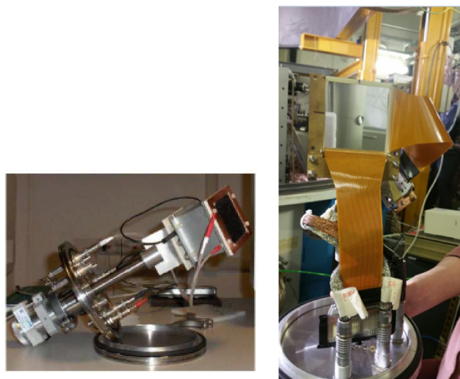
FIGURE 3.6: Left: Photo of the MCP detector mounted on a ISO-flange. Right: Photo of the DSSSD.
