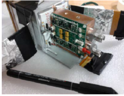
FIGURE 4.27: Copper block placed behind each telescope, in order to support and cool the four CsI(Tl) preamplifiers.
