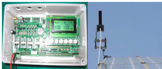
Figure 4: Tracker Control Unit (left) and Solarimeter (right).
