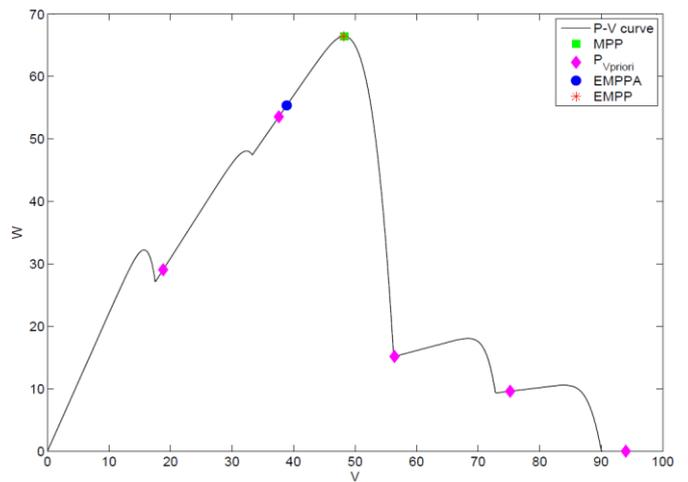
Fig. 5. The ANN discovers the correct "hill" but the amount of power wasted by EMPPA is not negligible.
