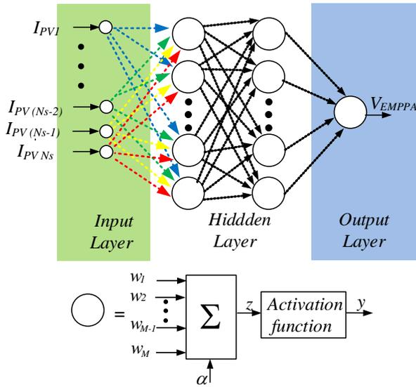
**Fig. 2.** Multi-layer feed forward neural network used for GMPPT.
