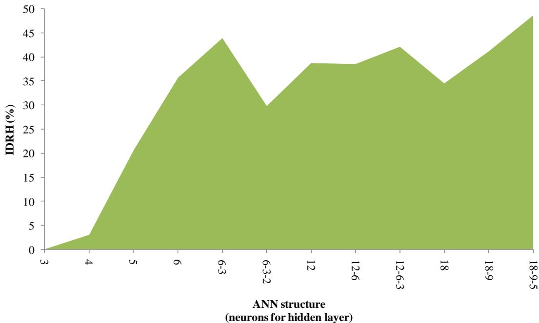
**Fig. 8.** Improvement in discovering the "hill" (*IDRH*) where the GMPP is located vs. ANN complexity.
