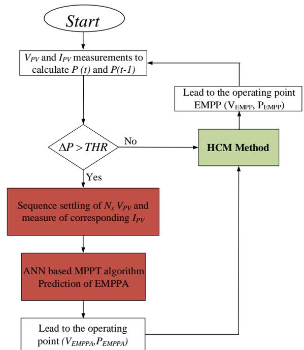
Fig. 1. Flowchart of the method coupling ANN with HCM.
