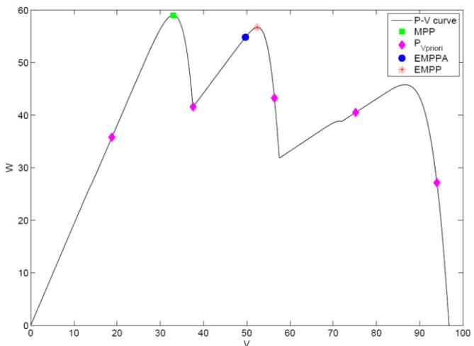
Fig. 4. The ANN fails in discovering the "hill" but the amount of wasted power is not large.
