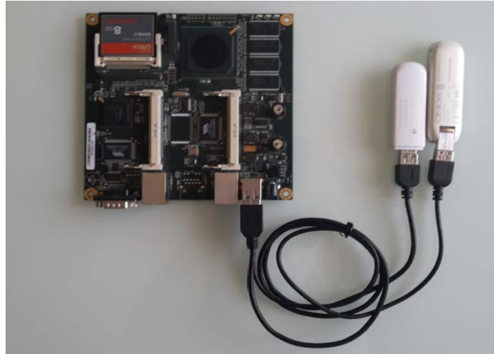
Fig. 7. The experimental prototype based on ALIX2D2 board employed during test campaign [2].
