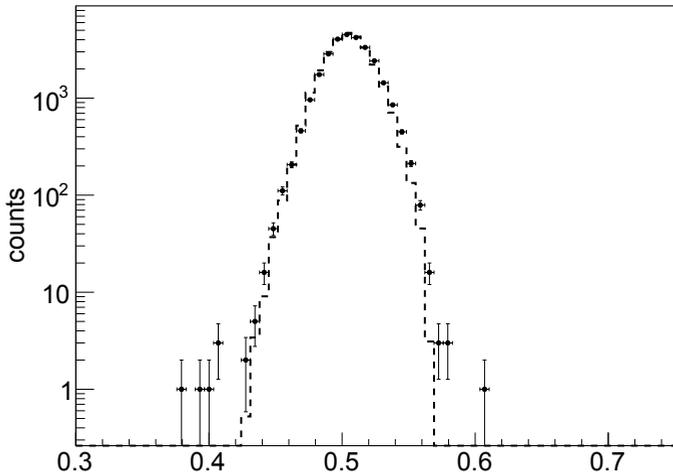
**Figure 4.** Distribution of the largest normalized energy  $\varepsilon_i$  in the decays of the Hoyle state. They are studied by means of invariant mass technique on experimental Hoyle state decay data measured in the hodoscope.
