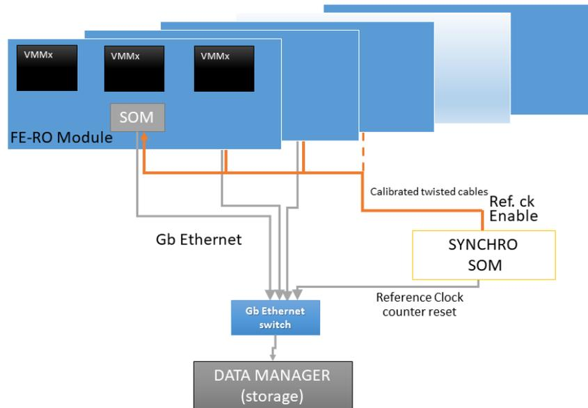
**Figure 2.** Architecture of FE-RO electronics and DATA Manager.
