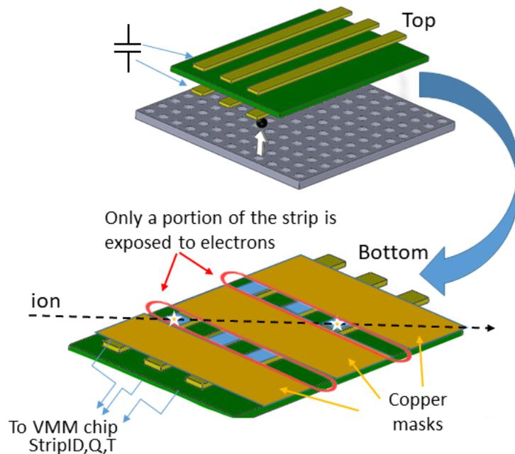
**Figure 1.** Schematic of the new FPD segmented anode board.
