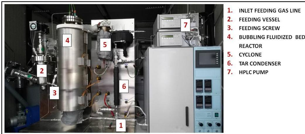
FIGURE 2. BFB bench-scale gasifier
