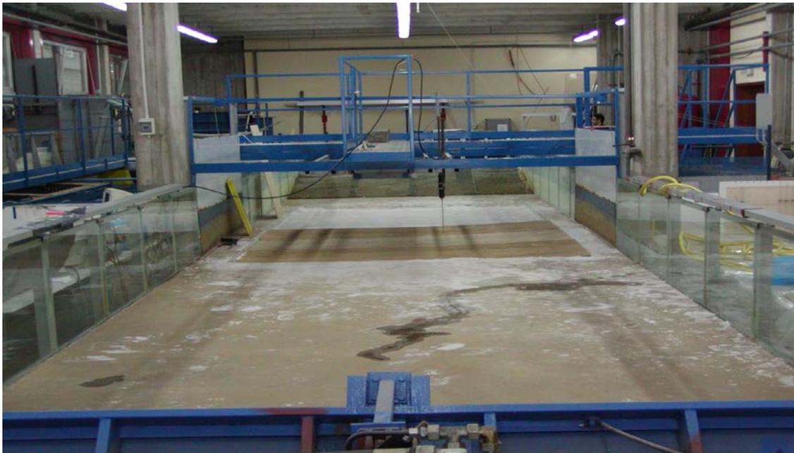
Figure 1 Picture of the experimental set up with the PVC rippled bed .
