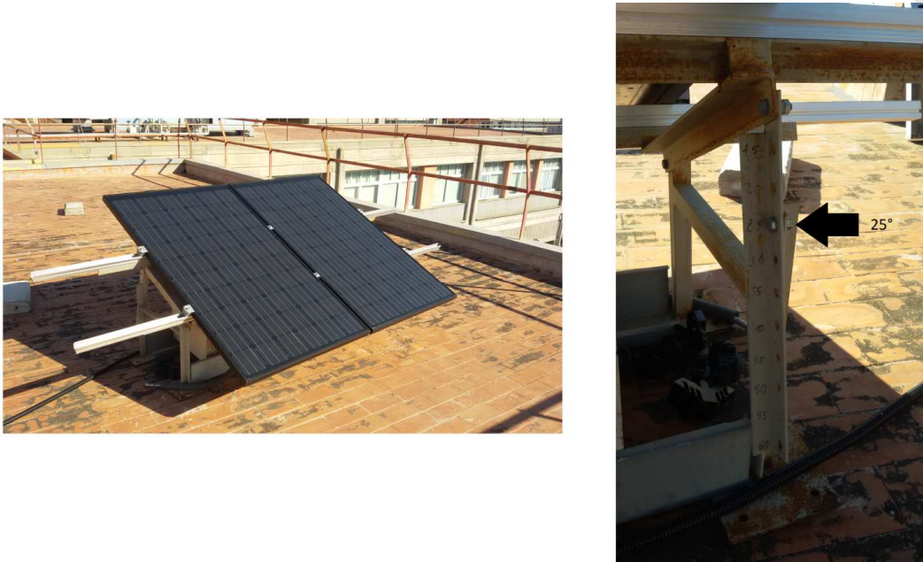
183 Fig. 1. Mounting structure: a) PV/T modules – b) Tilt angle setting structure, \beta .
